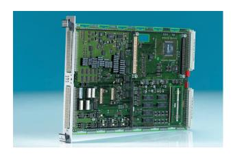
To control the switch matrix modules an IEC/IEEE bus interface is provided as standard. A high-speed TTL interface is available in the form of PC Card Interface PS-B11 from Rohde & Schwarz.
